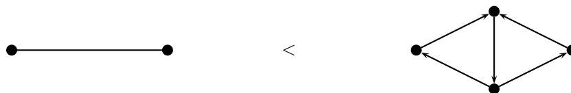
Figure 1: The undirected case is reducible to the directed case, using this gadget. Only one path can use these five arcs, either from left to right or from right to left.
